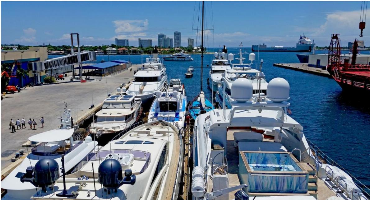
Superyachts settle into their berths aboard *Super Servant 4* during a recent DYT sailing from Port Everglades to the Med. \$350 million worth of yachts were loaded by DYT’s float-on method onto *SS4* and a second DYT ship, *Yacht Express*. Photo credit: Joseph Hoyt
